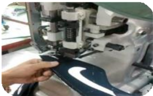
Hole punch & Eyelet attaching
